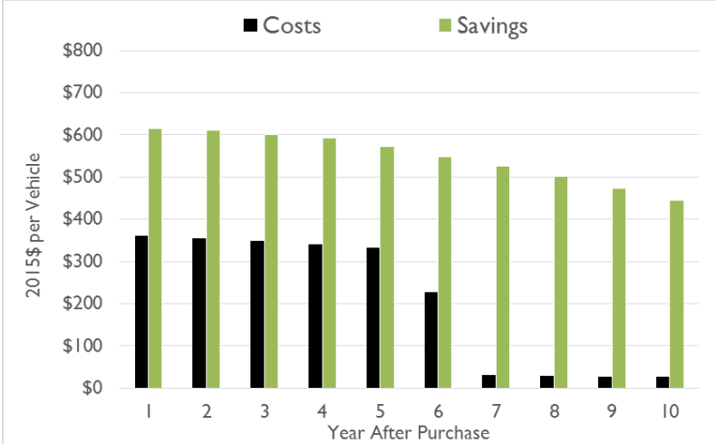
Figure 4: Annual Light Truck Compliance Costs and Fuel Savings (relative to MY 2016, assuming financing)
