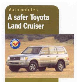
In recent years, the *Toyota Land Cruis*er has been reliable, comfortable, and quiet, scoring highly in most of our tests. But we couldn't recommend this large SUV because of its poor performance in our emergency-avoidance test, which simulates the vehicle's ability to steer around an obstacle in the road. Our test vehicle tended to spin out too easily in that test.
